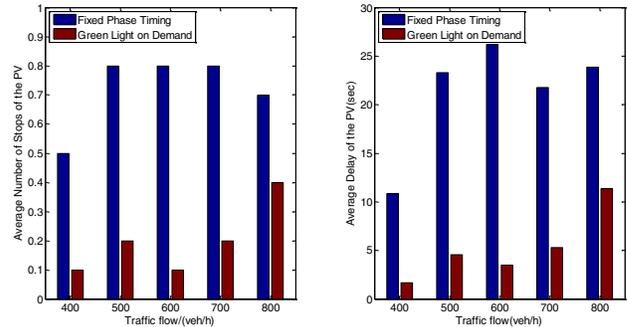
Figure 13. Average number of stops and delay of PV
