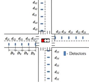
Figure 4. Detector Arrangement
