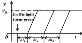
Figure 7. Velocity Curves during Starting Process
