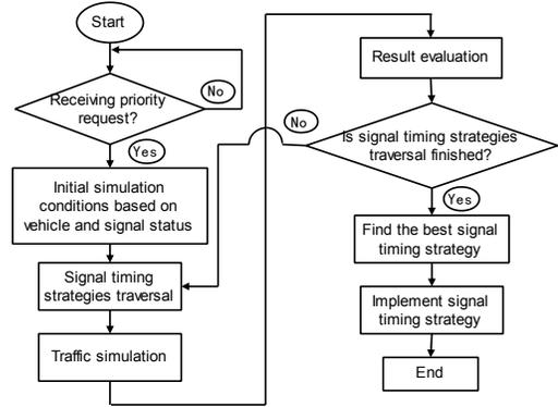
Figure 9. Flow Chart of Passing Algorithm based on Modeling and Simulation Method
