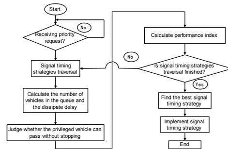
Figure 8. Flow Chart of Passing Algorithm based on Mathematical Analysis Method
