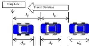
Figure 6. Space Relationship during Starting Process
