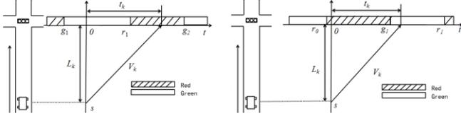
Figure 5. Condition for a vehicle to pass an intersection
