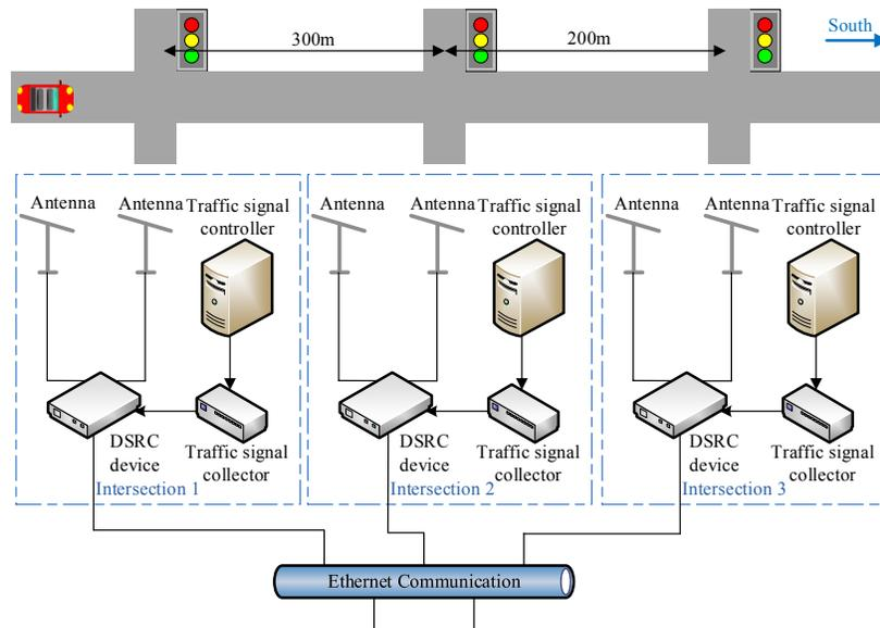
Figure 6. Schematic diagram of test bed
