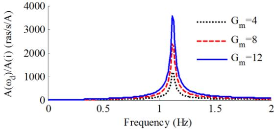
Figure 3. Amplitude ratio under different worm gear ratios\*
