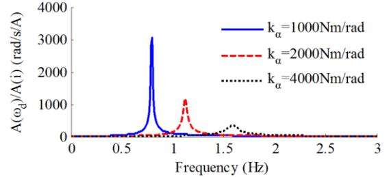
Figure 5. Amplitude ratio under different aligning stiffness\*
