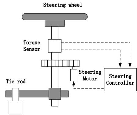
Figure 1. Schematic diagram of EPS (Ji-Hoon, K. et al. 2002)
