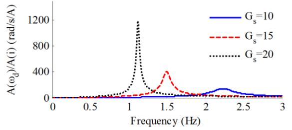
Figure 4. Amplitude ratio under different steering ratios\*
