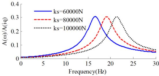
Figure 6. Resonance frequency of IWM\* (Chen, et al. 2016)
