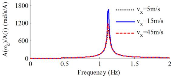
Figure 2. Amplitude ratio under different velocities\*
